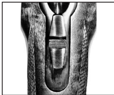
Figure 5. Safety selector in “FIRE” (full forward) position. The safety selector should be moved to this position only when the gun user is actually firing the rifle. If you choose not to fire, immediately return the safety to the “SAFE” position shown in Figure 4. (When the safety is in the “FIRE” position, it is referred to as being “off.”)
