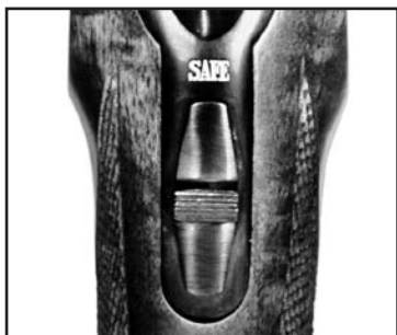
Figure 4. Safety selector in “SAFE” (full rearward) position. The safety selector should be in this position when the underlever is open to load a cartridge, or to unload a live round. Whenever a cartridge is chambered, the safety selector should be in the “SAFE” position unless the rifle is to be fired immediately. Keep the safety in this position except when actually firing. (When the safety is in the “SAFE” position, it is referred to as being “on.”)
